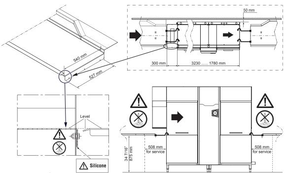
Apply silicone between the machine and the table and make sure that there are not any water leakages.
